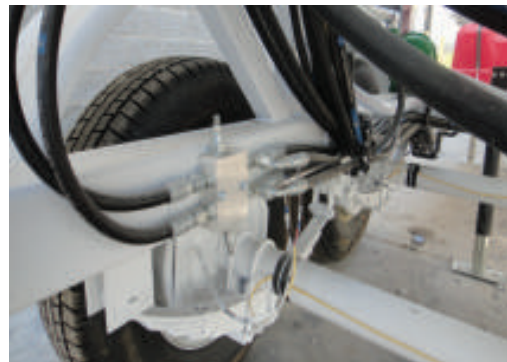
Full Hydraulic System runs off of the Diesel, Gas, or Electric engine.
