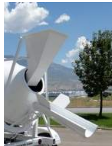
Gravity & Discharge Chutes
